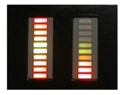
The monitor display is mounted to the right of the ignition switch as shown above on the left. A close-up of the display is shown on the upper right. The colors appear much brighter and crisper than the photo. The left column of Light Emitting Diodes (LEDs) is for the rear carb and the right column for the front carb. The leanest mixture is with all LEDs off. As the mixture becomes richer, lights begin to turn on from the bottom.
