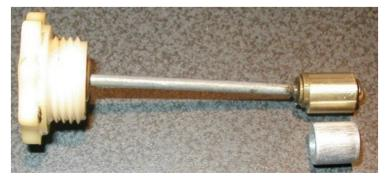
The photo above shows the damper with an extra piston beside it. If you look really close you'll see that the piston on the damper is longer than the original shown beside the damper. The original design allows 0.075 inch movement of the piston hence 0.075 undamped movement of the air valve. The original piston is 0.367" diameter, 0.375" long with a 0.200" hole. The replacement is .0370"
