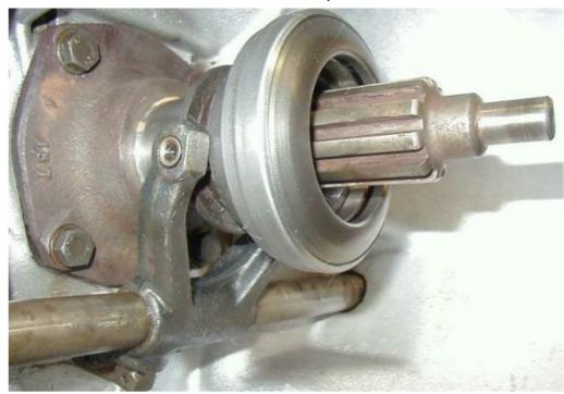
The next photo shows the gearbox front end cover and release-bearing sleeve (with bearing removed) in more detail.
