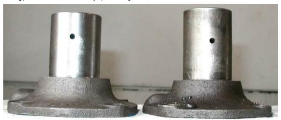
Murry's Fix: We decided to replace the front cover because of the depth of the scratches. We mounted another TR4 front cover in the lathe, cut off 3/8 inch, smoothed and rounded the end and then polished the outer surface.
