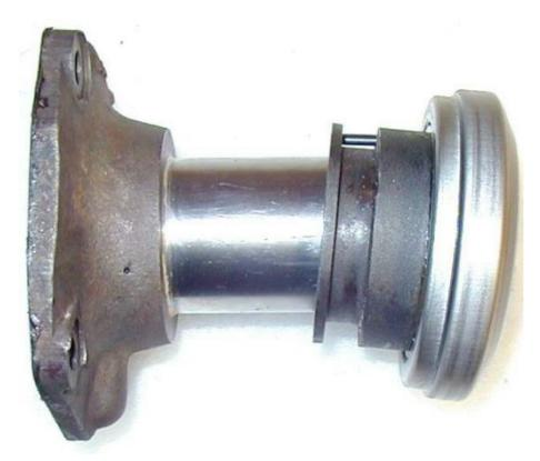
Some tilting of the sleeve is not surprising since the pins of the clutch fork sweep through the front end cover center line, but are either above or below the centerline during part of the sleeve travel. Also, the pressure plate is probably not aligned perfectly with the front cover. If the bearing aligns with the pressure plate, then the sleeve will be tilted. The fact that the sleeve hangs under the more than 200 lbs clutch pressure plate spring force is however surprising.
