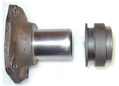
The front end cover outside diameter measured the same as one on another transmission and the same as those we measured last September. The sleeve inside diameter was then measured and the clearance computed to be .008 inches agreeing with similar used sleeves measured last fall. Thus, the problem wasn't a too small sleeve as I had suspected.
