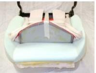
The upholstery is then pulled down over the front and sides and the small clips installed to hold it in place. I use a small hammer to drive the clips home. Bruce Miles had stopped over to observe the seat project and provided a lot of help with stretching and holding the upholstery as shown in the following photo.
