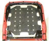
The back was next. (Those of you with sharp eyes will note that we're back working on the LH seat --- the first one.) I reinstalled the straps first and then sprayed adhesive on the areas of the back frame that contact the back foam and also on the matching areas of the foam. The bottom strap was also coated with adhesive. I then pressed the foam against the frame back --- see next photo.
