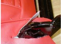
The rear flap was attached to the rear of the frame bottom next. The flap goes over the bottom half of the hairpin torsion bar. The upholstery was cut to accommodate the looped end of the bar as shown in the next photo (that happens to be of the LH seat).
