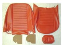
The two brown fiberboard stiffeners that fit in the bottom of the sides of the back upholstery are missing metal clips that must be removed from the old upholstery. The clips are held in place by split rivets that I was able to salvage with the clips. The two sides are mirror images as shown in the next photo.
