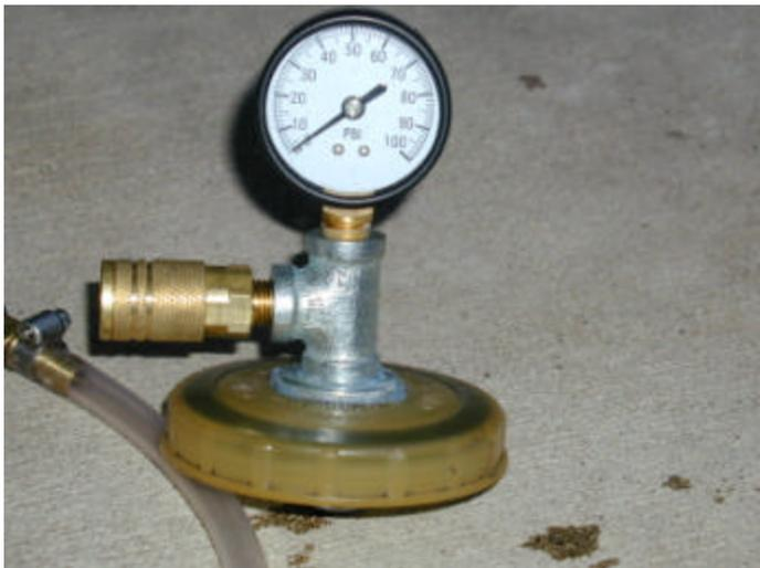
I used the quick connect setup to make it easier to take the cap on and off – in hind site I might have reversed the quick connect to keep the tank from leaking when we are all done.
