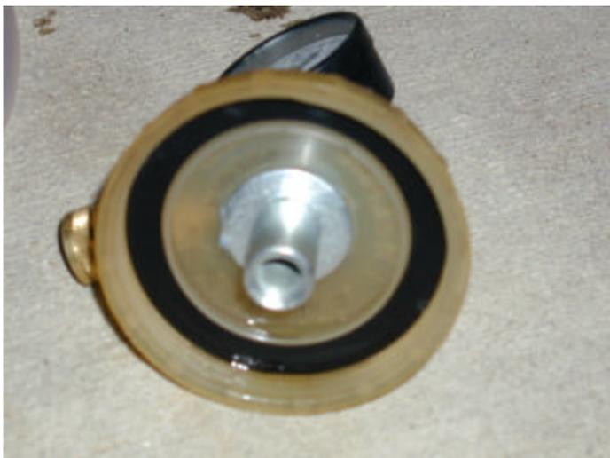
Inside the cap I places about a 1 inch coupling to tighten the washers to the cap, and it has the benefit of siphoning off extra fluid when we are all done.
