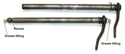
The major shaft wear points are where the back side of the shaft rubs against with the bushes. The photo below shows a heavily worn shaft that should be replaced.
