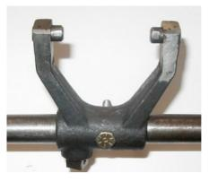
Note that the main pin should be inserted and tightened and then the fork and shaft drilled at the same time. I've noticed in several cases including the shaft - fork combination in the photo that the pin seats against the fork casting before the pin seats in the shaft hole. This may be caused by wear in the hole. In this case several new pins were tried with the same result. The cure is to grind about 1/8 inch off the top of fork boss under the head of the pin.
