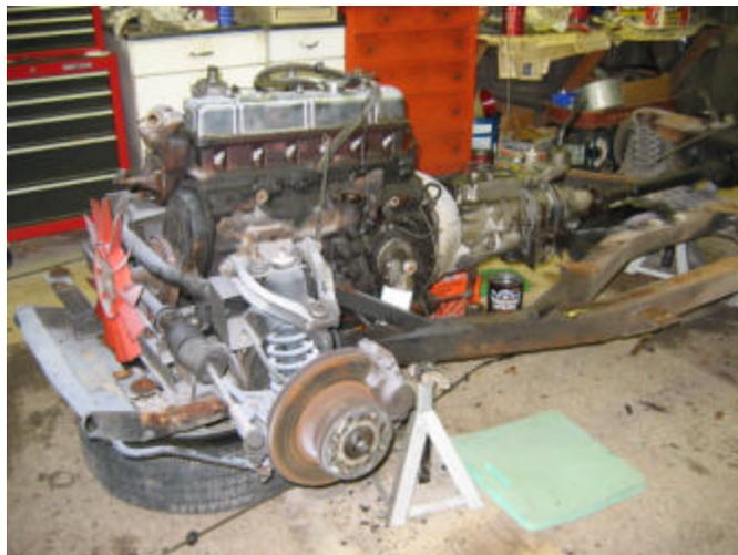
The item of real interest is the main differential bridge. Note in the picture the location of the springs in the end of the diff bridge.
