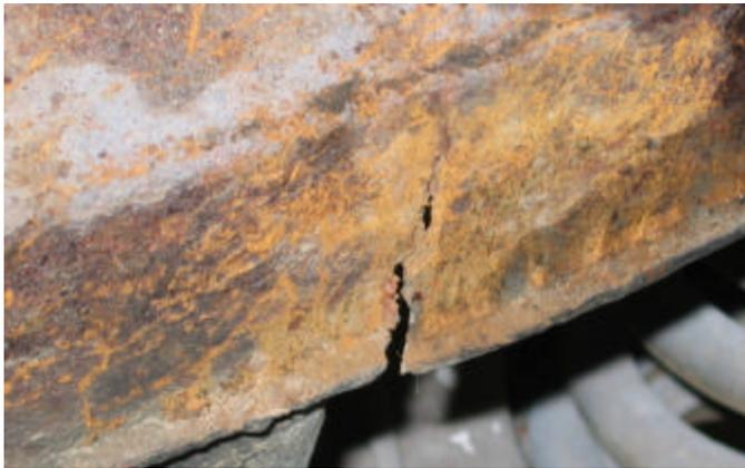
These cracks are big enough to stick a pretty good size nail in and they would surely have cracked across the top and allowed the spring to push the bridge against the tub.
