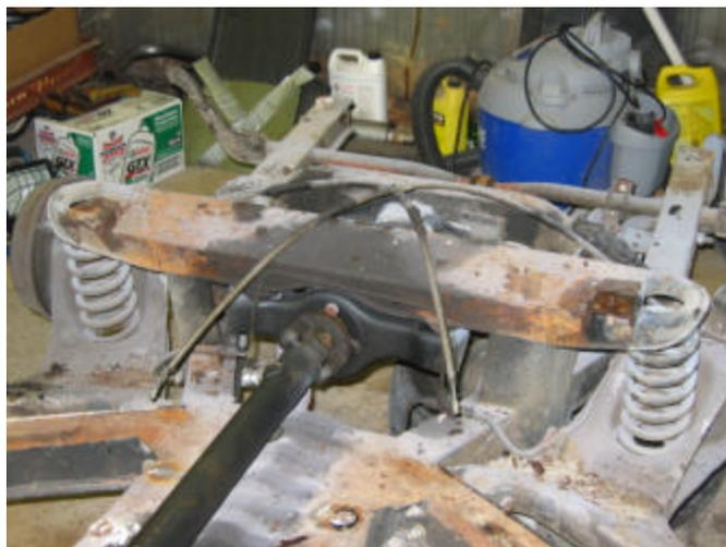
I found upon on closer inspection on the engine side of the diff bridge, cracks in the front part of the flange, which are caused by the pressure of the springs. I added stronger springs many years ago and this may have caused these cracks. Note the next two pictures.
