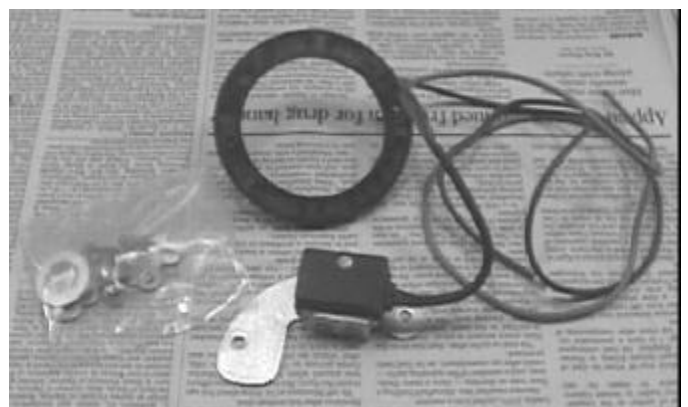
Petronix Kit For The GM Distributor: Pickup Unit Is In Front, Ring That Attached To The Weights Is In Back
