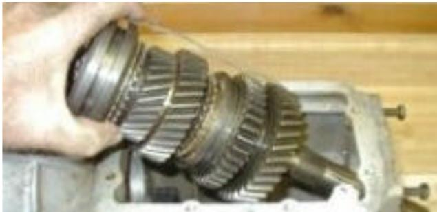
The outer ring of the third and fourth speed synchro hub is moved to the rear most position --- engaging the third speed gear. This is done to provide clearance with the front most countershaft gear. The mainshaft is then positioned as far forward as possible without interfering with that front most countershaft gear.
