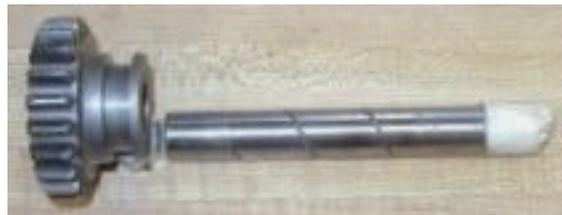
The end of the shaft is wrapped with masking tape to prevent it from moving too far forward during the assembly process. The next photo shows the interior of the gearbox at this point. The masking tape on the reverse operating lever holds the reverse idler gear as far forward as possible to keep it out of the way during the rest of the assembly process. The countershaft is then removed so that the
