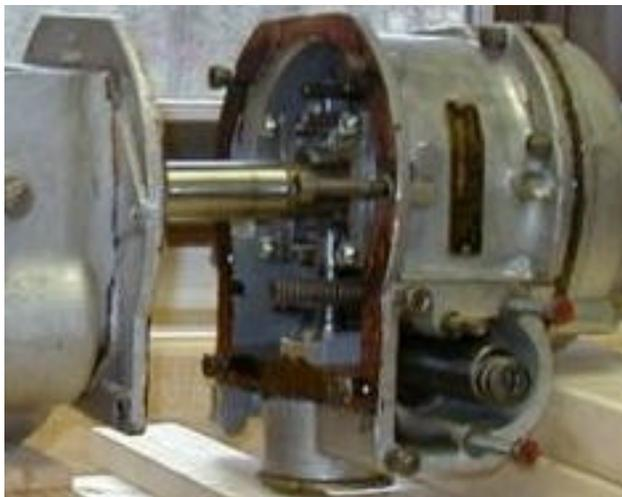
**Installing Rear Extension (Non-OD Gearbox)**
