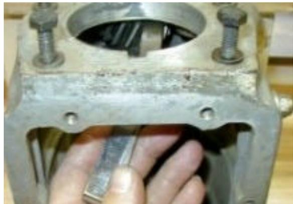
Next, the gearbox is returned to the horizontal position and the reverse idler gear and shaft installed, making sure that the gear engages the reverse operating lever (that was not removed during disassembly). These components are shown in the next photo.
