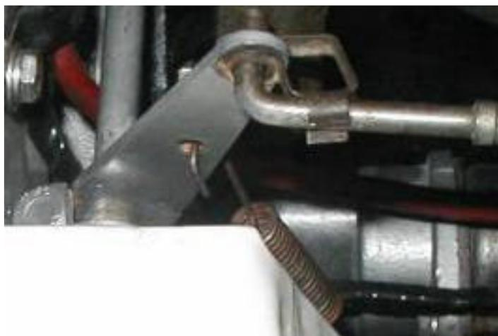
The next step was to loosen the nut on the control lever pinch bolt and try to slide the lever off the shaft. The lever wouldn't slide off mine so I placed a piece of plastic between the end of the shaft and the bulkhead and then drove the lever off using a long screw driver & hammer as shown next photo.
