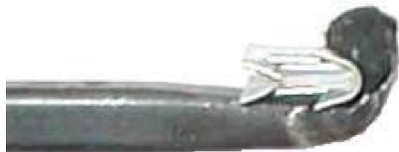
The tool is merely an old screwdriver with the end bent over to form a hook. Some sticky body sealer is placed on the hook to retain the clip. A clip is then placed in the hook and the tool with clip is slid into the window gap at the top front of the door and then worked into position where the clip is to be placed. The tool is then lifted up forcing the clip over both the lip on the outer door panel and the door waist seal.
