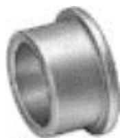
*An alloy of copper, tin, and carbon, these porous sintered bronze bearings are vacuum-impregnated with 18-20% SAE-30 oil. Heat created by shaft movement draws the oil to bearing surface. The oil acts as a cushion between the shaft and bearing, reducing wear and increasing resistance to shock loads.*
