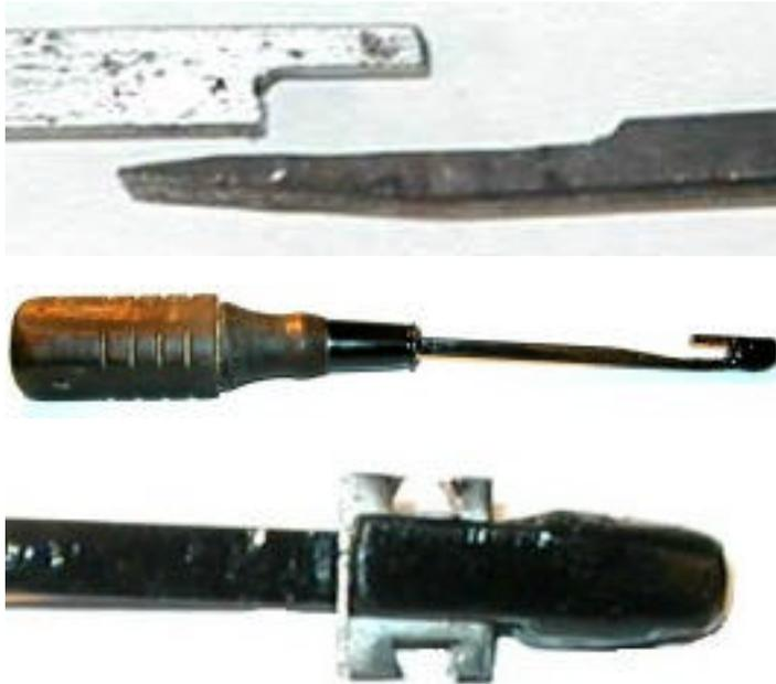
The clip extends beyond each side of the tool and the little barbs on each side of the clip near the edges keep the clip from sliding off the side of the tool; no more lost clips. Further, the tool can be slid on an old clip still on the door lip and the clip can then be pushed down and off the door lip with a screwdriver. The clip will be retained in the tool for easy removal and later reuse.
