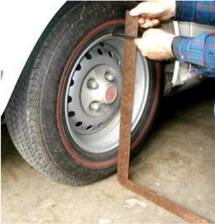
First and most important, all tires must be inflated to equal pressure and the car pushed unoccupied to the place of measurement. If the car had been turned or worse, the back end jacked up and then put back down, the suspension will not be at equilibrium because the bottom of the tires are restrained from moving in or out by the floor.
