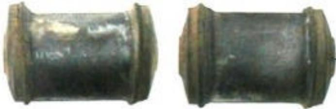
If the bushes are more than ten years old I'd suggested replacement before doing anything to adjust the camber. The standard bushing as well as up rated rubber and poly bushes are available.
