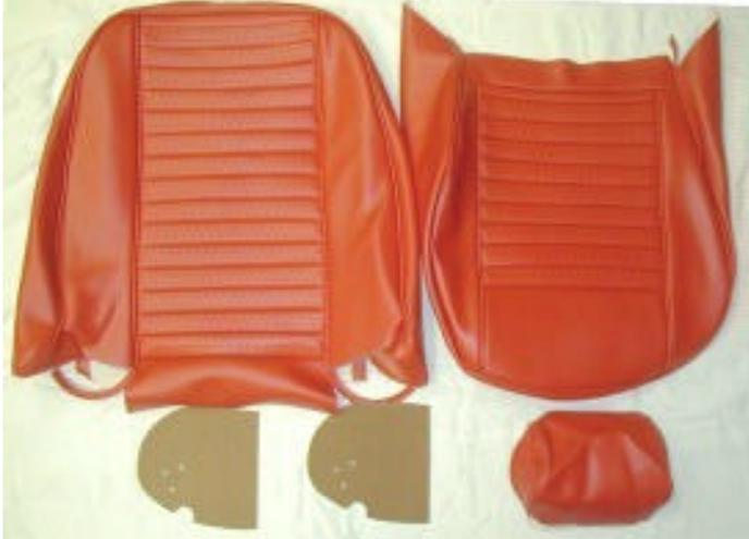
The two brown fiberboard stiffeners that fit in the bottom of the sides of the back upholstery are missing metal clips that must be removed from the old upholstery. The clips are held in place by split rivets that I was able to salvage with the clips. The two sides are mirror images as shown in the next photo.
