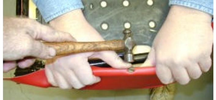
The final step on the bottom was to trim the upholstery in the area where the tubular clips go in the rear and then cement the upholstery in place. The tubular clips were then installed to hold it in place while the adhesive dried. The under side with clips installed is shown in next photo.
