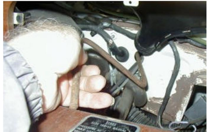
The tool is positioned properly when the middle segment is horizontal and the other two segments are nearly vertical. The vertical segment in the engine compartment should rest against the hood release lever as shown in following photo.
