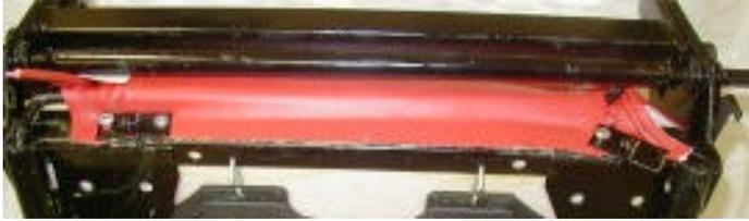
Next, the cloth strips on the under side of the seat upholstery (one at front and one on each side) were cemented to the seat bottom foam – see next photo. The long strip at the front was stretched over the front and held while the adhesive set.
