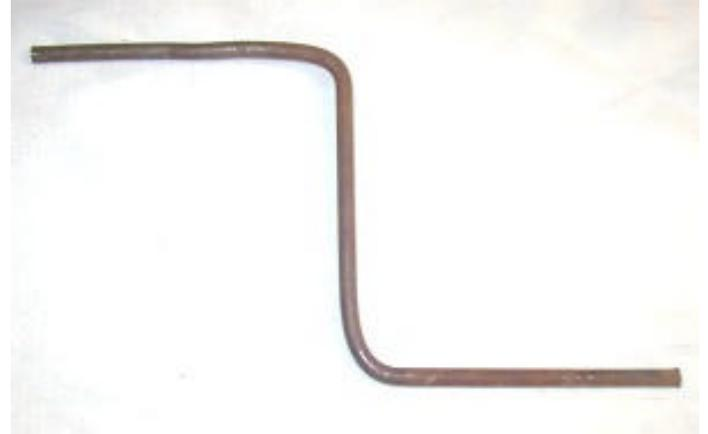
The stay under the glove box, the glove box, and the right side ventilation ducts are removed. The rubber grommet in the hole through which the temperature control and choke cables pass is pushed forward into the engine compartment. The tool is then inserted into this hole; see next photo.
