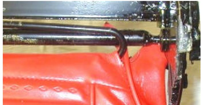
Adhesive was sprayed on the underside of the rear flap and the mating frame surface. I then used a sharp punch to pierce the upholstery for the control rod bracket screw holes and screwed the brackets into place – see next photo. These served to hold the back flap in position while the adhesive dried and later when the upholstery was stretched over the front. I took a break at this point to allow the adhesive to dry.
