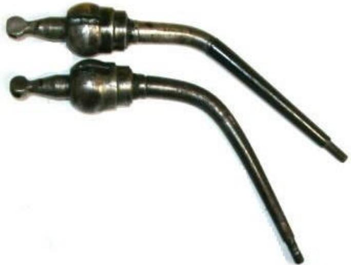
When the top cover was disassembled, signs that the 3<sup>rd</sup>/4<sup>th</sup> selector shaft been forced past the interlock were found. I suspect that someone tried to force the gearbox into reverse while it was still locked in 3<sup>rd</sup> or 4<sup>th</sup> either through the incorrectly set selector or the bent fork prong. It then went to work chewing up the reverse gear teeth.
