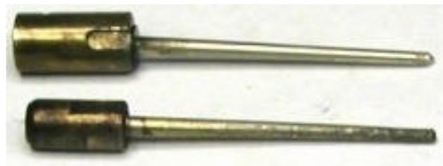
**Needle Recess:** Careful inspection of the fixed needle air valve revealed that if the needle recess were enlarged and the closed upper portion drilled out, this area of the two valves would be identical. Of special importance is that the position of the shoulder where the lower side of the lip on the adjustment screw rests is the same in both the adjustable needle air valve and the fixed needle valve.
