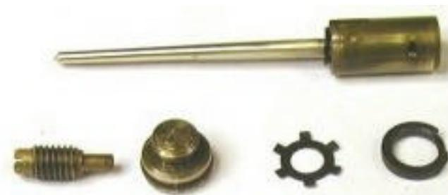
The photo above shows the adjustable needle with needle retaining screw, adjustment screw, adjustment screw retaining clip and an old damaged O ring that fits in the slot on the adjustment screw. The photo below shows a comparison of the adjustable needle with the larger carrier and the fixed needle with the smaller carrier. The actual needles are identical.
