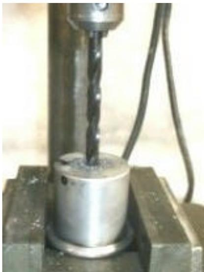
The photo on the left shows drilling out the needle recess with a Letter O drill (0.316 inch). A 5/16 inch (0.312) was tried first but the hole was too snug for the needle carrier. The adjustment screw slid down into the valve from the top with no problem. A 5/16 inch steel rod was used to tap the retaining clip into position. The needle also slid into position with no problem. These were
