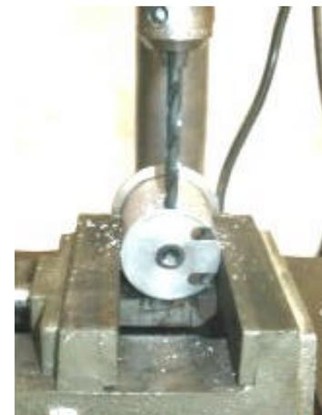
Next, a lathe was used to fabricate an aluminum plug. The plug outer diameter was turned to 0.224 inch. The center was drilled 0.159 inch with a Number 21 drill and the plug was cut to ~ 0.3 inch length. The plug slid in the first ~0.3 inch depth and then encountered resistance. The plug was then driven into the final ~0.3 inch with a punch.
