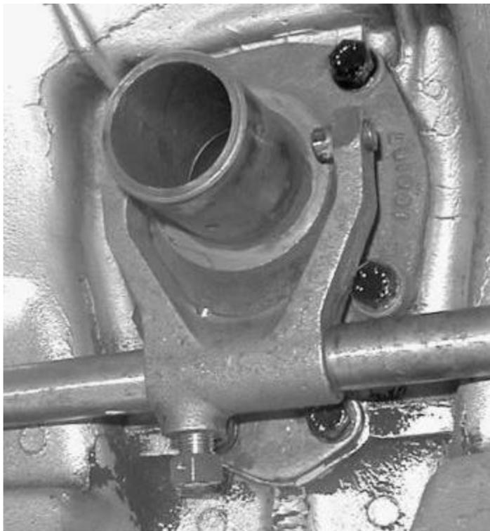
Clutch fork with pin installed. Photos are of a transmission case that the throw-out bearing and main shaft have been removed for clarity.
