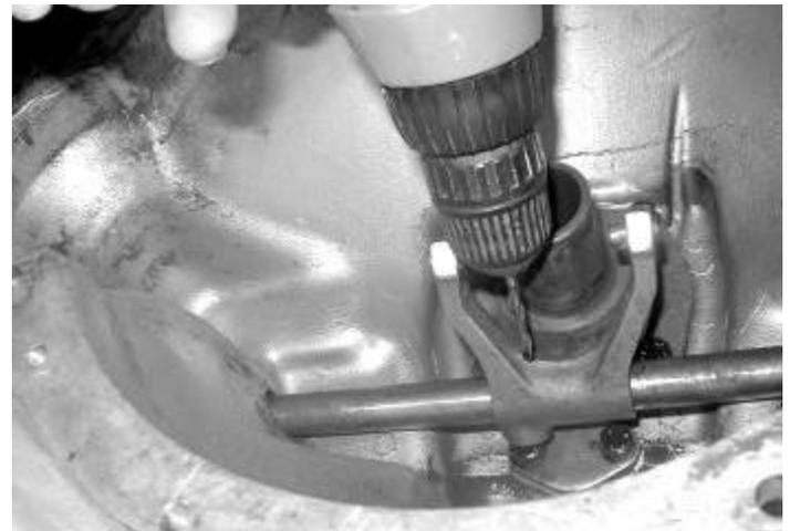
Drilling hole in clutch fork
