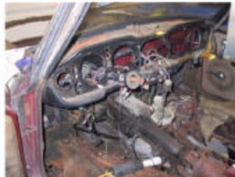
I have completely removed all the gauges etc so the dash is completely stripped now, even removed the heater box .. I even took apart the ignition switch.. (springs went everywhere)
