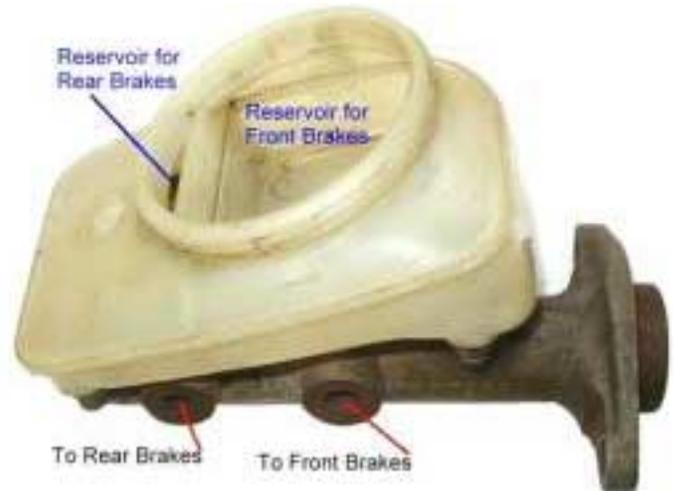
The master cylinder internal components are shown in the next photo. The system uses tandem pistons. Although it's not obvious from the picture, the primary piston is a little larger diameter than the secondary piston. The primary piston pushes the fluid to the front brakes as well as pushing fluid to drive the secondary piston that supplies the rear brakes; hence the primary piston does double duty. Aren't these parts filthy? They really clean up nice as seen later.
