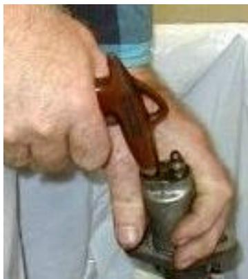
bottom. Next, push the air gun into the input port on the cylinder and trigger the air as shown in photo. In most cases the piston will fly out, especially if the cylinder has been in use recently.
