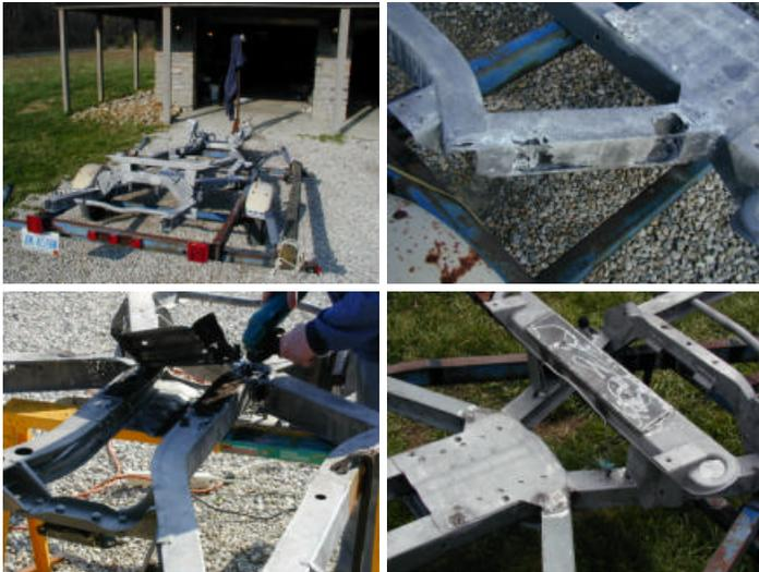
With much help from Nelson Riedel we were able to weld in a new cruciform (center plate) and new trailing arm mount cross members. We also reinforced the mounts for the differential. To finish everything off with a nice touch we painted everything in a nice epoxy primer and topcoat.
