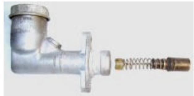
The cylinder inside surface is inspected to make sure it is clean and smooth. There is usually some corrosion near the open end of the cylinder. As with the slave cylinder, this area is beyond the travel area of the seal and can be readily cleaned with steel wool. I've never seen a damaged master cylinder so in most cases no honing is required. If honing is
