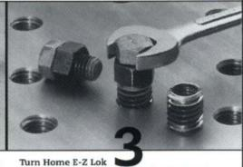
Use bolt as illustrated to install E-Z Lok. Nut prevents hang up of E-Z Lok on grip of bolt. Use two nuts locked against each other to shorten bolt to proper thread length.
