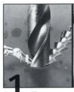
Drill Drill hole according to table on back. E-Z Lok can be used in extradeep or through hole.
