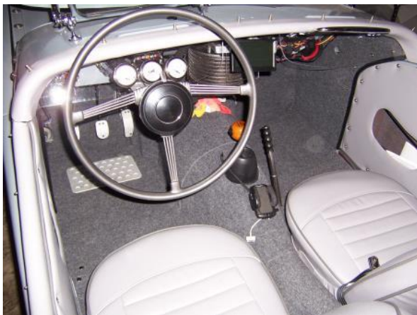
New Plexiglas Dash(s) – the gauges float
