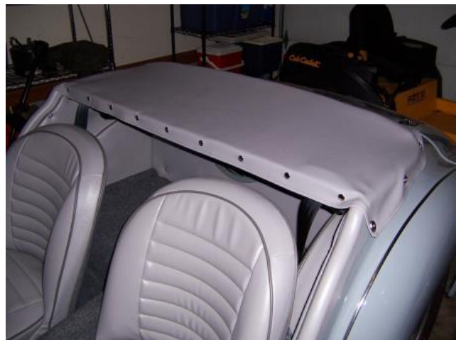
The back cover – yes, I still have the tonneau to seal the interior up.
