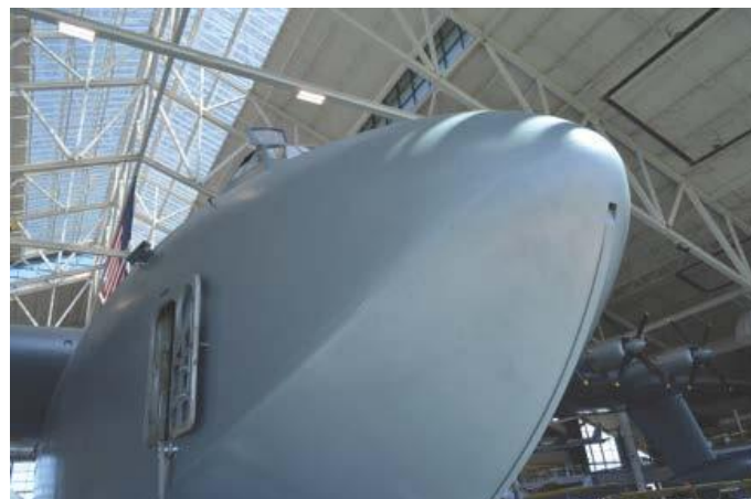
They used laminated birch due to steel being in short supply
