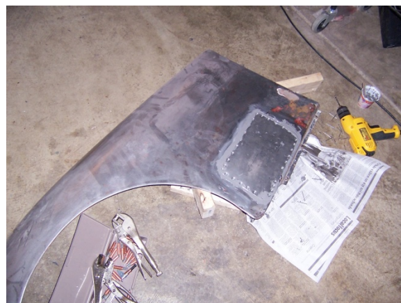
Patch in place.
