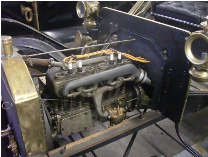
Ford Model S engine (Notice choke cable out to crank)
