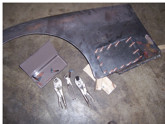
Patch panel in place before attachment
