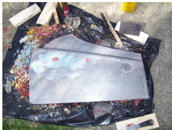
Driver's Door after stripping - old paint and filler is to the left.
