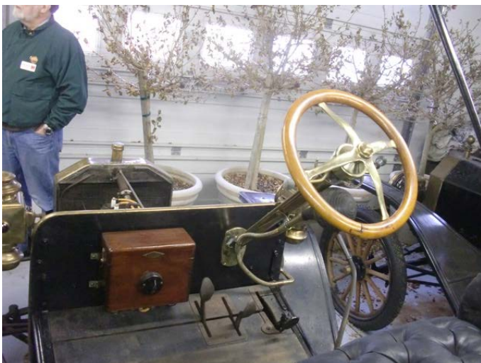
Model S dash. Wood box is 4 coils triggered by crank switches. Column accelerator.
