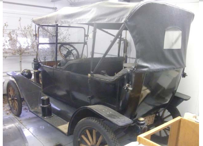
Model T (teens maybe) Prestolite gas generator tank on running board to power headlights
