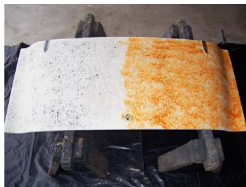
Methylene chloride-based stripper on the left, citrus on the right, 15 minutes into the experiment
