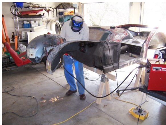
Mike McK welding away at some stress cracks
