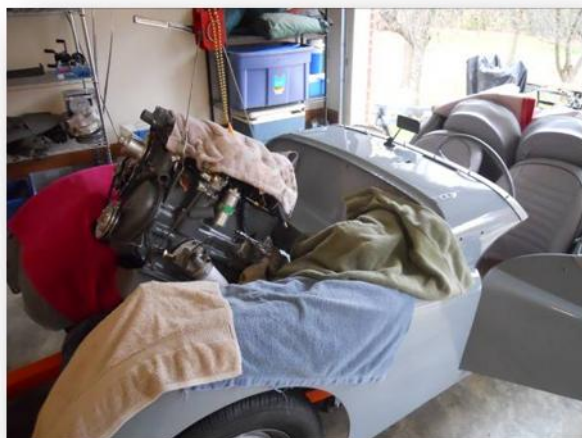
Going back in – note the increased insertion angle needed
