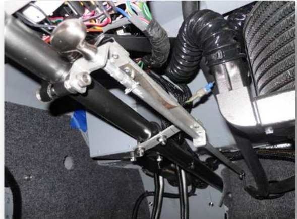
Choke mechanism mounted on the steering column
