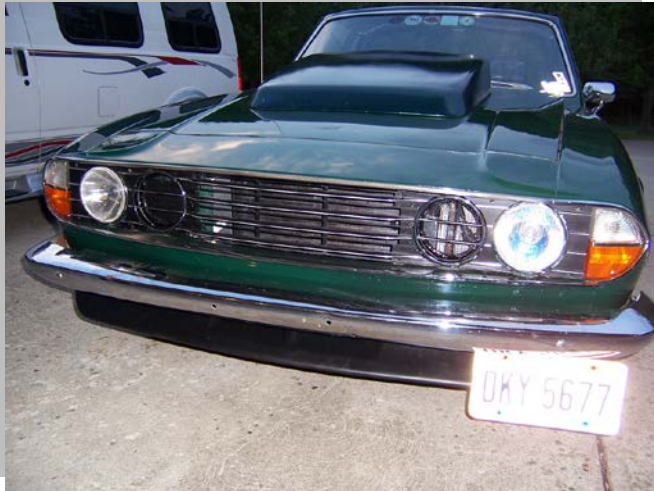
Inner headlights replaced with air vents way back when...how about that hood riser???
