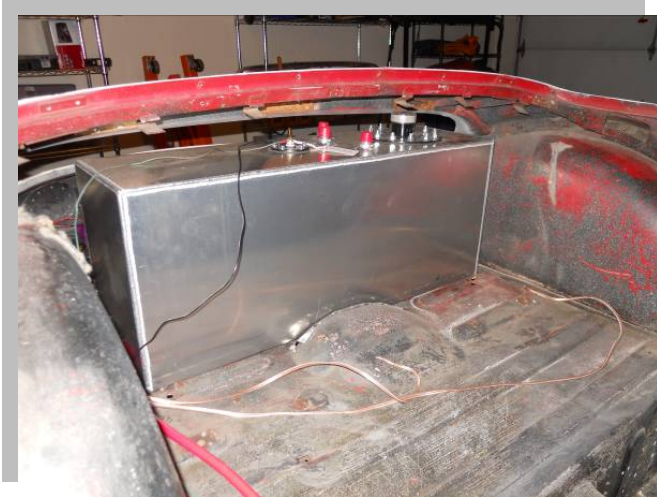
New fuel cell in place
