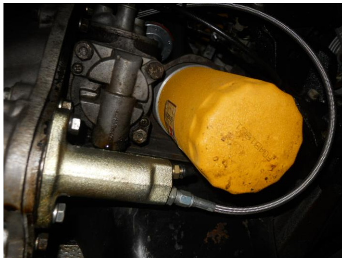
See, oil pump area! Yes, that is a spin-on filter.
