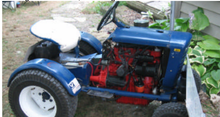
A garden tractor with an engine from a Mini.
