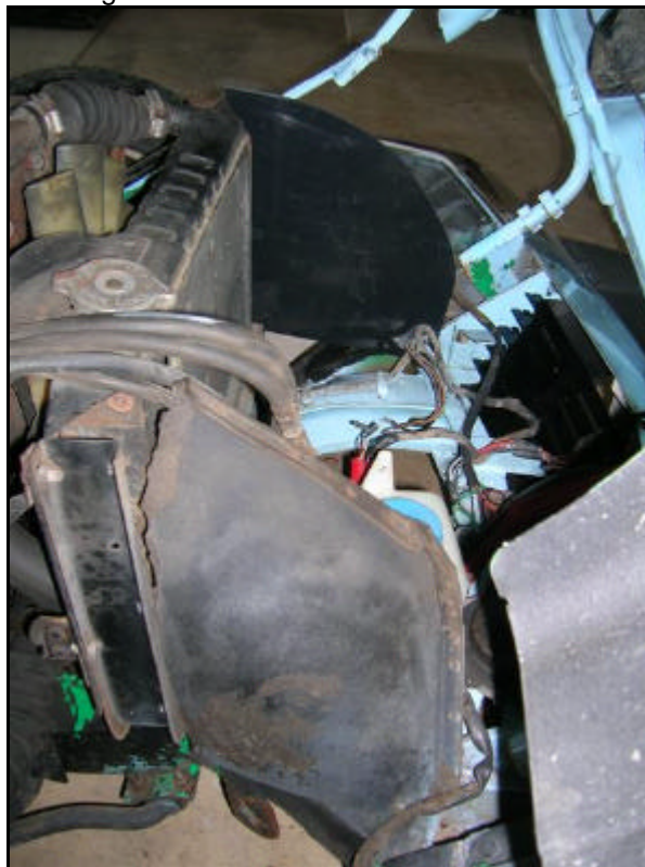
Test fit the new deflector. Note the condition of the right hand deflector.
