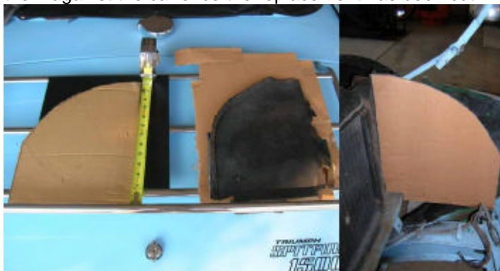
Create the template from the original deflector (if available). Test fit to verify that alignment and clearance is correct.
