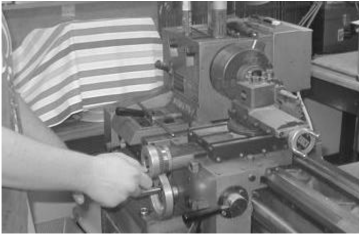
Ryan trying to bore sleeve --- it didn't work either
