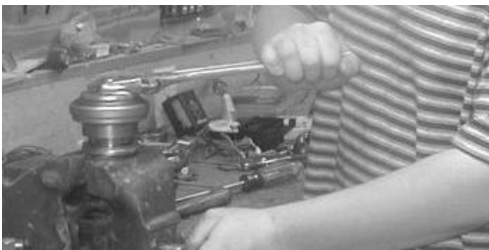
Ryan pressing on new bearing using TRF tool.
