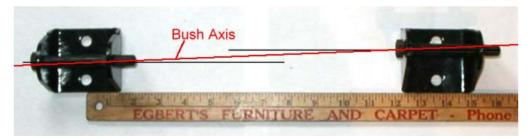
The angle (in radians) between the bracket centerline and the bush axis is approximately equal the difference in the bush bolt positions of the two brackets divided by the distance between the center of the brackets (13.635"). The angle can be converted from radians to degrees by multiplying by 57.3. I defined a positive angel as the case where the inner BBP is above the outer BBP. Combining all this, the Bush Angle is approximately:
