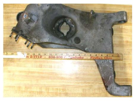
The first thing is to get our directions straight. If the bush axis is raised, the front of the trailing arm goes up and the back goes down resulting in raising the car and increasing the positive camber. If you draw a couple sketches you'll see that the car height changes 10.5"/19" or 55% of the change in the bush axis height.
