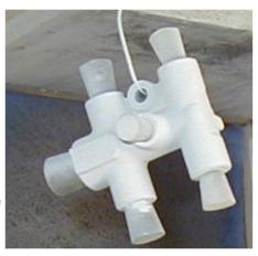
In most cases the objects are wired below an oven rack that is hung from one of the rotating hooks for painting. The rack and parts are then transferred to the oven for curing. The next photo shows master cylinders and hydraulic pipes ready for PCing.
