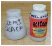
The adapter was made by cementing the lid (center cut out) of an Eastwood cup into the top of a HF cup. When using the Eastwood cups on the HF gun, the cups should be no more than 1/3 full. The cups that are supplied with paint are about 2/3 full. The excess powder can be stored in small plastic bags for later use.
