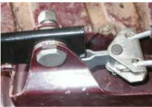
The outer cables were then slid over the notches in the bracket. If there is insufficient cable slack, the pins attaching the fork end to the rear wheel cylinder lever can be removed and then reinstalled after the outer cable has been positioned.
