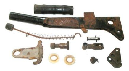
Some of these parts are obviously in worse shape than those of the '76 handle. For example, the '70 paw release knob has a hole as shown on the right. Won't speculate as to why handbrake was applied with such urgency to make the hole. I decided to use any part from the later lever assembly that was the same as for the early lever assembly and in better shape. (I also have a '76 so wanted to keep the unique '76 parts.)
