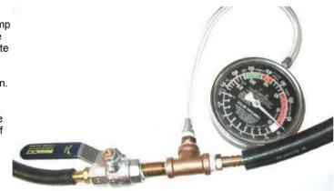
**Bench Test:** The first thing I did was to plug the hose and determine the maximum depression I could create --- 21" Hg. I then closed the valve to determine how long it could hold it ---- slowly bled down (or I should say up) to half the starting depression in 2 minutes. After checking around I figured out that one of the pipe fittings was leaking slightly. Fixed that and it held the depression
