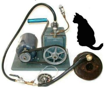
This shows the plumbing in more detail. The valve is between the pump and the servo. This allows the hose to the pump to be sealed and the rate of depression loss observed. The gauge is a compound gauge that reads both pressure and depression. Another setup will be to supply compressed air at a low pressure, close the valve and observe the rate of loss of pressure as an indicator of the non-return valve health.
