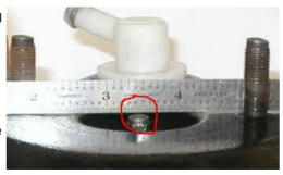
While I don't have specifications for the push rod adjustment I can make some guesses. We don't want it too short to avoiding introducing slack into the system. We don't want it too long because it might prevent the primary piston from returning far enough to open the tipping valve. The 0.035" gap that moves the primary piston about 0.005" off the stop seems to be reasonable.
