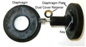
The valve assembly is retained in the diaphragm plate by a little key that is visible after the diaphragm has been removed. The key is easily removed by pushing the pedal push rod in and
