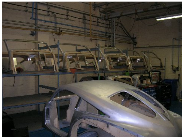
A stack of Aero 8 bodies and an AeroMax body shell waiting for production.
