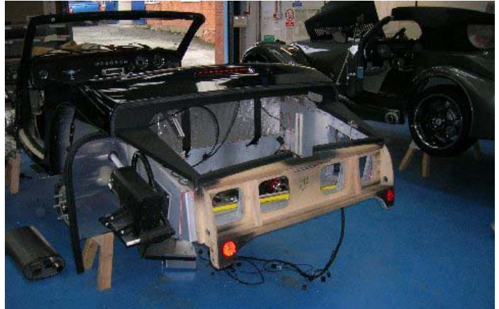
Note the relocated fuel tank creates a larger storage area in the boot.
