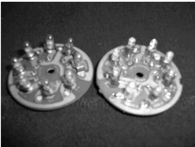
Original Idiot Light Cluster Bulb Holder On Left, One With LEDs Installed On Right. Not Shown Is The Idiot Focusing The Camera & Taking The Photo...
