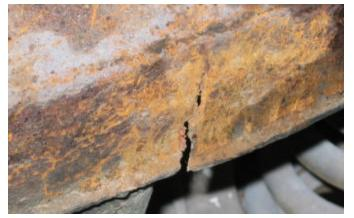
These cracks are big enough to stick a pretty good size nail in and they would surely have cracked across the top and allowed the spring to push the bridge against the tub.
