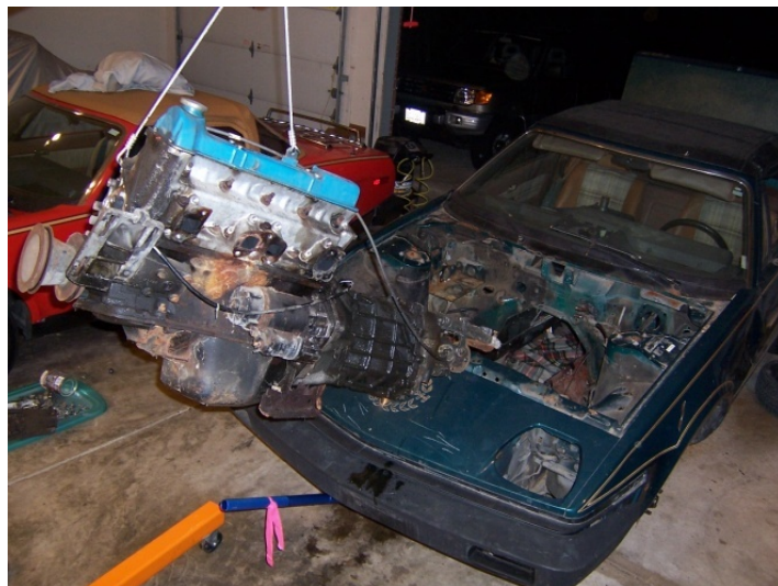
One engine out of the car – kids do not try this at home. Not shown is the radiator fluid all over the floor – forgot to plug the fitting on the back of the head – ooops!
