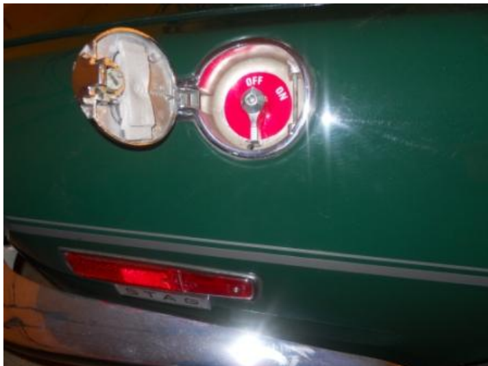
Hey look Ma, found the perfect place to put the battery disconnect switch!
