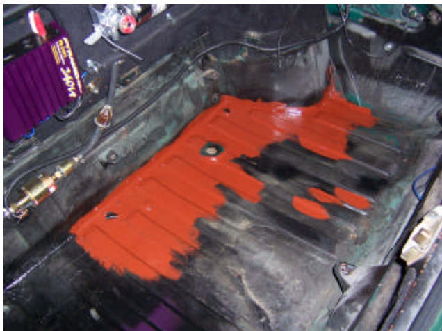
Figure 2: Trunk Floor Being Dealt With
