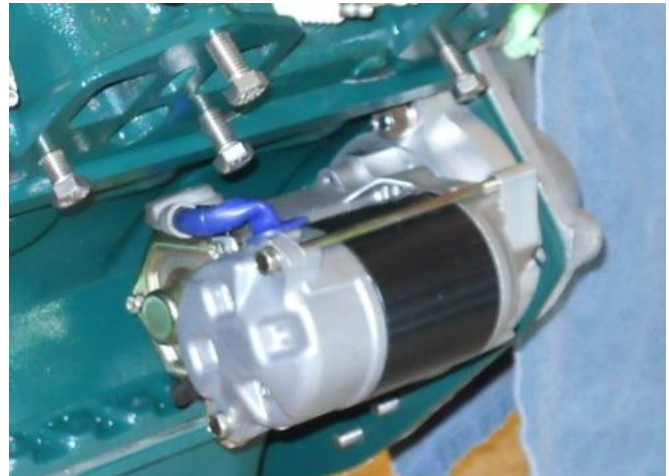
Starter motor in place on the block
