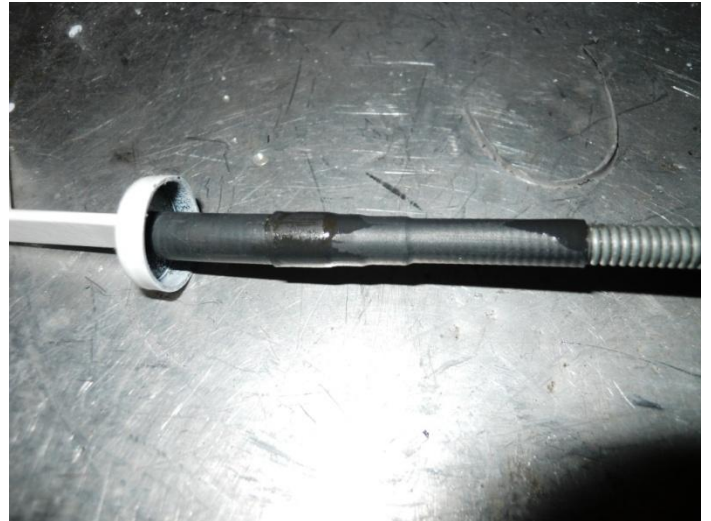
Dip Stick covered with shrink tubing – you are right, it's a lame subject for a photo, but it's my column...
