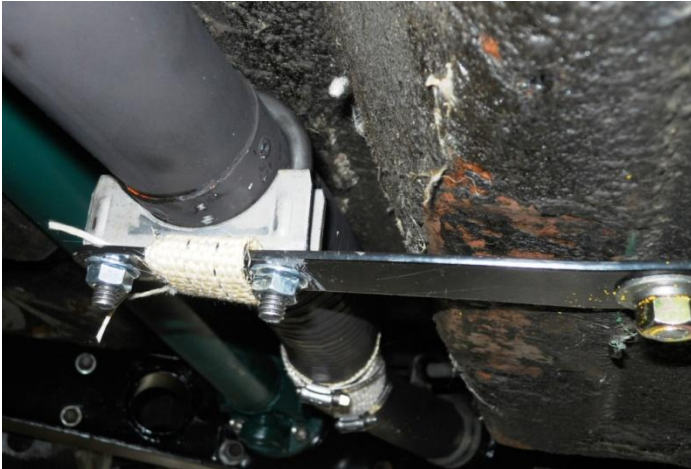
Middle brace. Note that you could take this across to the other side of the car so it could act as a drive shaft support in case of shaft failure. I'll note that for a future upgrade...
