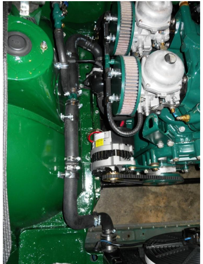
Hose run from block, through pump, reverse direction and head toward radiator – note that this is the opposite direction of the actual water flow – now that's confusing...
