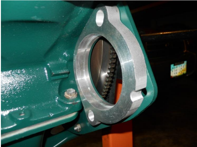
Spacer placed on engine – engine casting part that causes the interference is just to the left.
