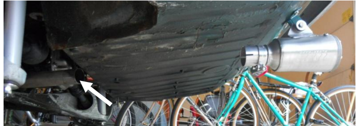
Muffler and pipe in place on the FrankenStag – white arrow shows the end of the pipe that goes through the back sub-frame.
