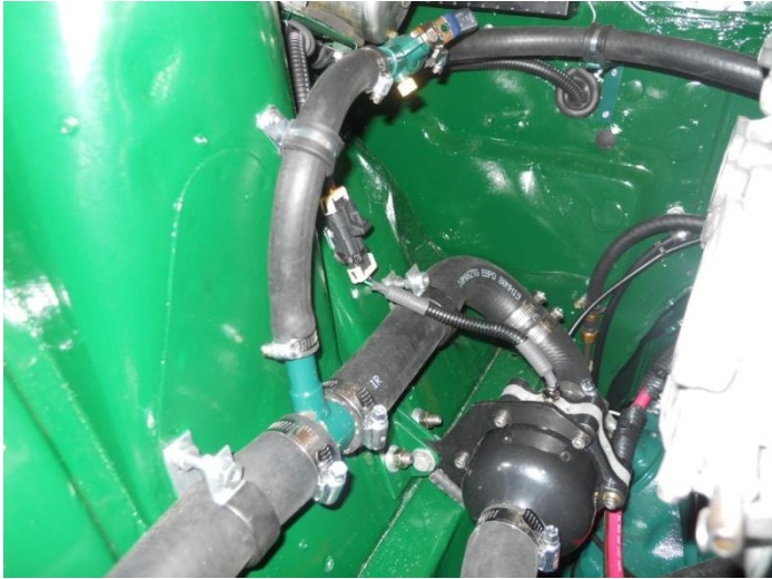
The “T” connection where the heater return line joins the radiator line headed back to the pump.
