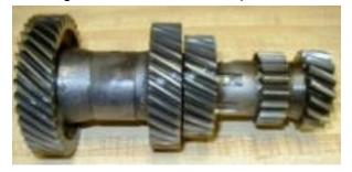
Countershaft Gear Installation
