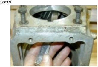
leveling it off with a file. This brought the end float into
