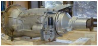
The previous photo shows the assembled gearbox. The only thing missing is a couple switches in the top cover and the wiring harnesses for the backup light and for the OD solenoid. They're around here someplace --- unless the spouse threw them out.
