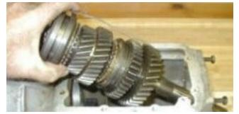
The outer ring of the third and fourth speed synchro hub is moved to the rear most position --- engaging the third speed gear. This is done to provide clearance with the front most countershaft gear. The mainshaft is then positioned as far forward as possible without interfering with that front most countershaft gear.
