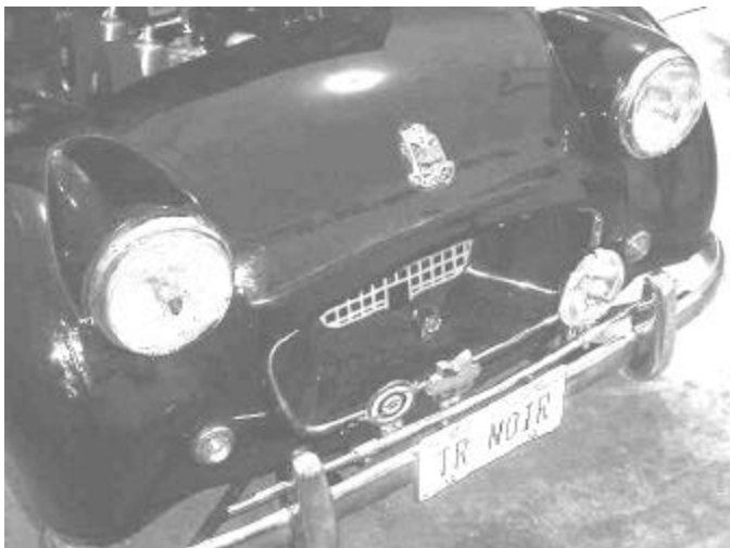
Daytime driving lamp on badge bar – remember when I said I wouldn't do this?
