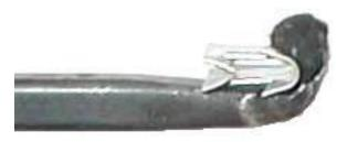
The tool is merely an old screwdriver with the end bent over to form a hook. Some sticky body sealer is placed on the hook to retain the clip. A clip is then placed in the hook and the tool with clip is slid into the window gap at the top front of the door and then worked into position where the clip is to be placed. The tool is then lifted up forcing the clip over both the lip on the outer door panel and the door waist seal.
