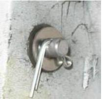
shaft and the side of the control were marked so that the control lever can be reinstalled in the same position. The next task was to disconnect the control rod from the control lever, remove the spring attached to the control lever, slide the shaft towards the left and slip the washers off the end of the shaft.
