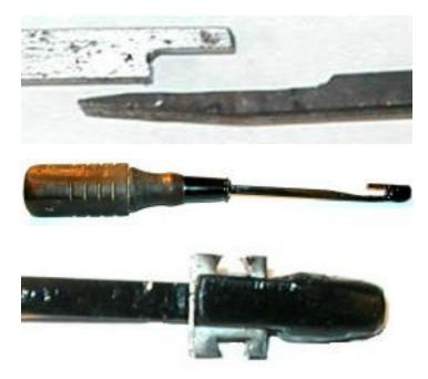
The clip extends beyond each side of the tool and the little barbs on each side of the clip near the edges keep the clip from sliding off the side of the tool; no more lost clips. Further, the tool can be slid on an old clip still on the door lip and the clip can then be pushed down and off the door lip with a screwdriver. The clip will be retained in the tool for easy removal and later reuse.
