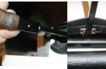
There's the tool in action with a clip just moved into position. Note that I seem to have placed the clip a little off center of the recess in
