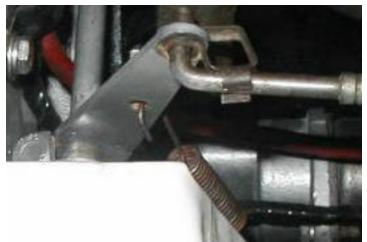
The next step was to loosen the nut on the control lever pinch bolt and try to slide the lever off the shaft. The lever wouldn't slid off mine so I placed a piece of plastic between the end of the shaft and the bulkhead and then drove the lever off using a long screw diver & hammer as shown next photo.
