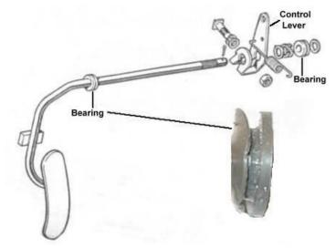
Removal of the shaft is no big deal, pull the cotter pin and loosen the nut on the bolt squeezing the control lever so the lever will slide off and then withdraw the lever through the driver's side.
