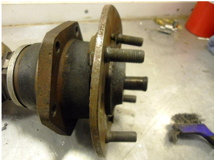
...bent hub and smashed threads on the other...
