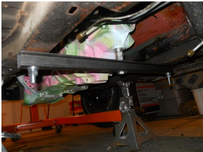
Conan – the back tranny mount! Bring me your women! See how visible that engine/trannie is with the high-viz paint scheme?
