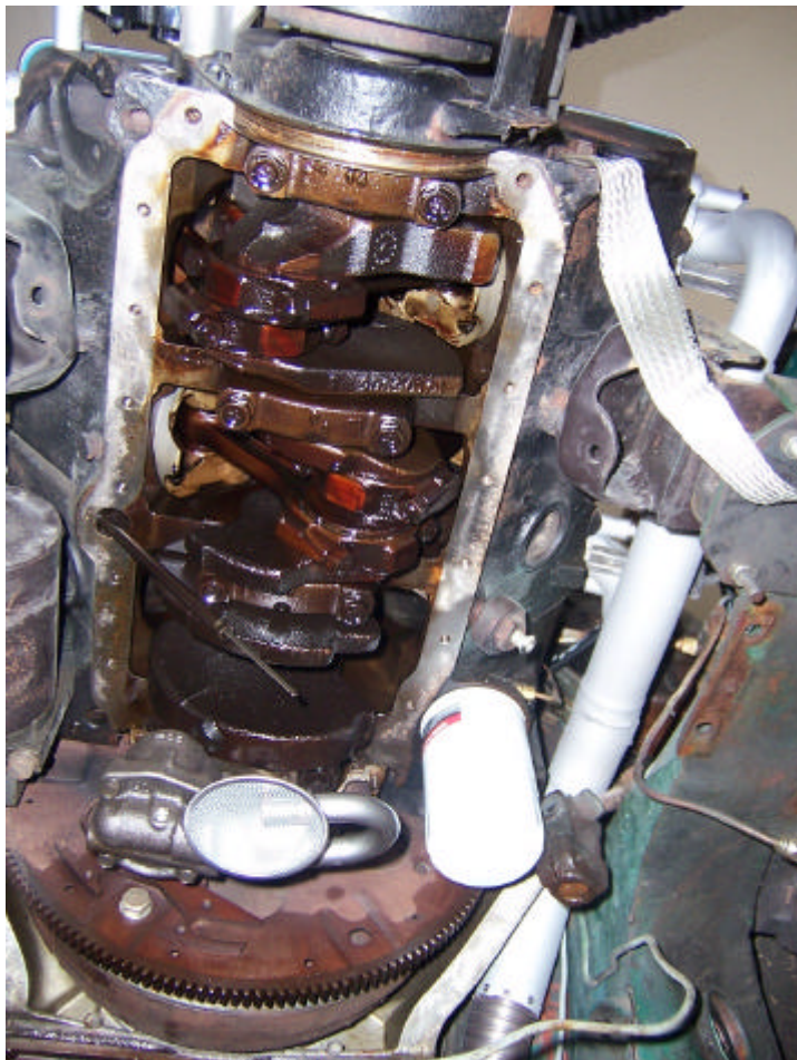
Engine With Its Pants Down – Trial fit of a new oil pick-up
