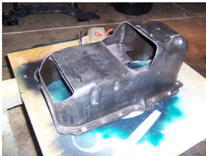
Oil Pan Modified To Clear Front Suspension w/o Lift Kit
