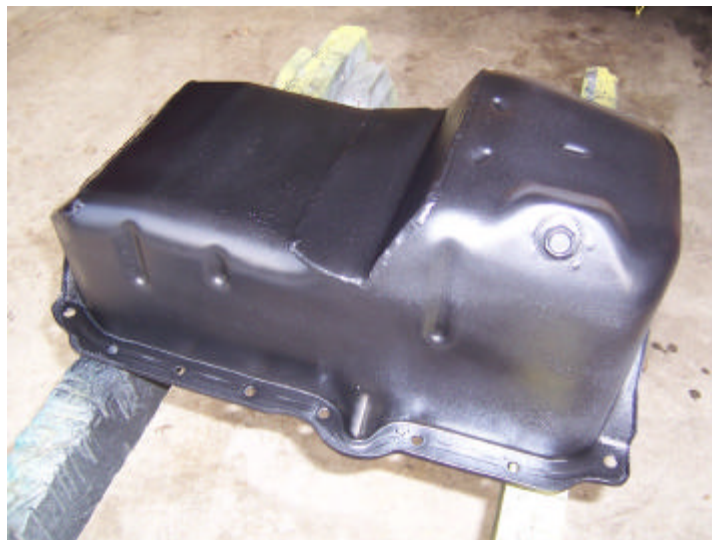
Modified Pan Ready To Put Back On
