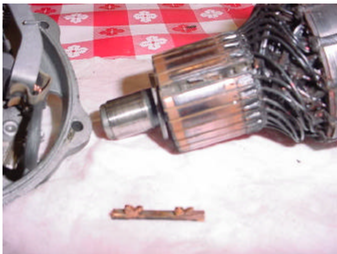
Commutator segment and the place it came from
