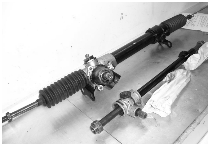
Old Power Rack In Back, Manual Rack In Front
