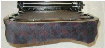
The seat bottom foam pad was installed next. I sprayed the top of the frame around the outer edge and a half inch strip around the outer edge of the under side of the foam. The sides of the pad are beveled resulting in the top surface being bigger than the bottom surface (that's how you tell which side is top & bottom). The next photo shows the installed pad.
