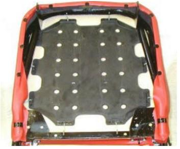
The back was next. (Those of you with sharp eyes will note that we're back working on the LH seat --- the first one.) I reinstalled the straps first and then sprayed adhesive on the areas of the back frame that contact the back foam and also on the matching areas of the foam. The bottom strap was also coated with adhesive. I then pressed the foam against the frame back --- see next photo.
