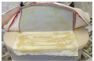
Next, the U shaped edge roll was cemented into place on the bottom foam over the cloth strips attached in the previous step as shown in next photo.
