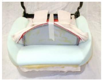
The upholstery is then pulled down over the front and sides and the small clips installed to hold it in place. I use a small hammer to drive the clips home. Bruce Miles had stopped over to observe the seat project and provided a lot of help with stretching and holding the upholstery as shown in the following photo.
