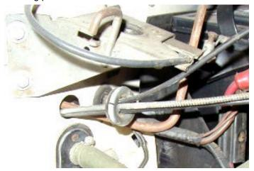
The hood is released by pushing the bottom of the tool to the left causing it to rotate around the middle segment and
