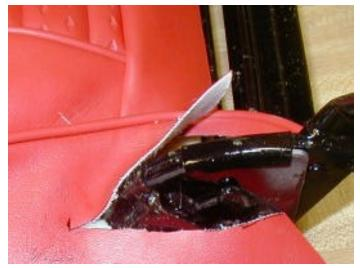
The rear flap was attached to the rear of the frame bottom next. The flap goes over the bottom half of the hairpin torsion bar. The upholstery was cut to accommodate the looped end of the bar as shown in the next photo (that happens to be of the LH seat).
