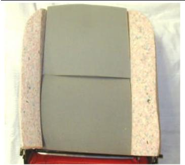
While this was drying I inserted the fiberboard stiffeners into the back upholstery. The original upholstery had these stiffeners stapled to the upholstery. I decided to just let them ride in the pockets at the bottom of the sides. I trimmed around the clips to ease attaching the clips to the frame.
