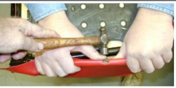
The final step on the bottom was to trim the upholstery in the area where the tubular clips go in the rear and then cement the upholstery in place. The tubular clips were then installed to hold it in place while the adhesive dried. The under side with clips installed is shown in next photo.
