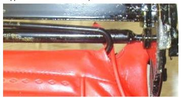
Adhesive was sprayed on the underside of the rear flap and the mating frame surface. I then used a sharp punch to pierce the upholstery for the control rod bracket screw holes and screwed the brackets into place – see next photo. These served to hold the back flap in position while the adhesive dried and later when the upholstery was stretched over the front. I took a break at this point to allow the adhesive to dry.
