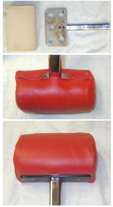
The angle control arm was polished and installed together with the headrest to complete the job. The finished product is shown in the last photo.
