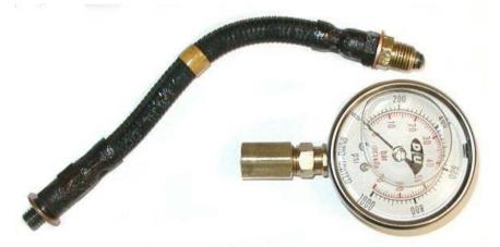
The gauge is shown connected to the OD in photo on right. The gauge reads a little less than 200 psi. I must have had the unit spinning and up to full pressure and then stopped the spinning but left the solenoid operated --- the pressure then must have bled down to the pressure noted. (Yes, if you look carefully, you see the clip leads from the battery are still connected to the solenoid.)
