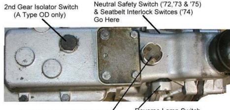
3rd & 4th Gear Isolator Switch ( Both A & J Type OD) **Reverse Lamp Switch**
