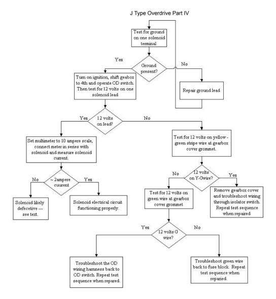
If the circuit passes the test in the flowchart I would then verify that the voltage on the solenoid goes to zero when either the ignition or OD switch is turned off or when the gearbox is shifted to neutral or any gear other than 3rd or 4th. If this doesn't happen, then the switch that doesn't affect the voltage should be examined.
