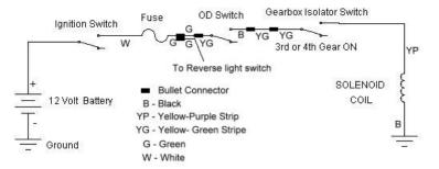
The OD electrical is powered from the **White** ignition wire, the same wire that goes to the ignition coil. After the fuse it becomes the **Green** circuit that powers the wipers, instrument voltage stabilizer (temperature & fuel gauges) heater fan and turn signals. The physical wiring configuration is:
