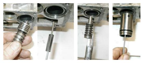
**Relief Valve:** The dashpot piston slides out easily after the valve plug as been removed, left photo above. The center photos above show removing the residual spring with a hooked wire and the valve with pliers. The dashpot sleeve is removed by slipping the hook at the end of the wire through the little hole.
