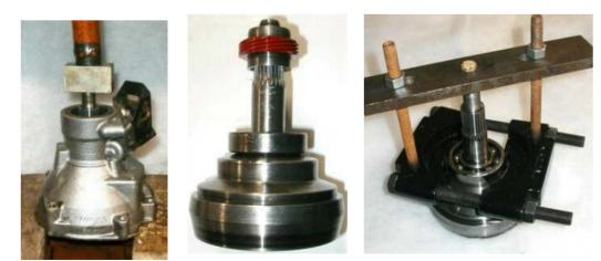
**Rear Seal:** I don't know an easy way to pull the rear oil seal. The best way I've found is to use a hammer and chisel to deform the seal enough so that it can be pried out with a screwdriver as shown on the right. The rear annulus bearing left in the casting when the annulus was pressed out can be removed after the rear seal is out. I tapped the bearing out from the inside of the case using a long pin punch on the outer race.
