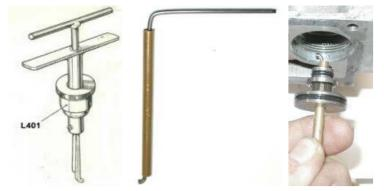
**Pistons:** The pistons were pulled out easily using pliers as shown on the right.
