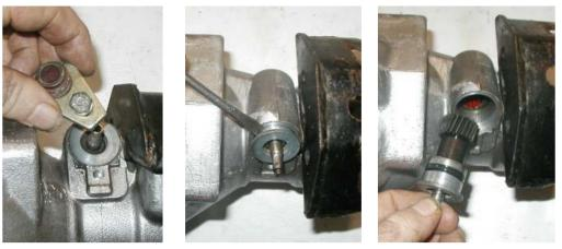
**Rear Flange:** The instructions say use a RG 421 tool to retain the flange. Looked in the toolbox and couldn't find anything labeled RG 421. I did however have a long flat steel bar with a 5/16 hole drilled in the end ---- just the ticket. After the nut was removed, the flange slid right off.
