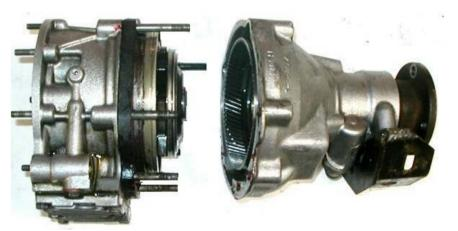
The photo above shows the separated castings. The planet carrier with planet gears came off with the main casting and sun gear. It was held there by friction between the sun gear and planet gear teeth. It some cases it might stay in the annulus. Care should be taken that it not fall off the bench
