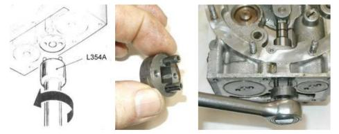
**Pump:** The right photo above shows removing the pump plug. This plug was much tighter than the other two plugs. The casting had to be held securely to break the plug loose. The piston and cam combination was removed after the plug was removed (it can be removed before too). I pushed the pump body out from the top with a finger as shown on the left below.
