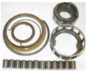
**Annulus:** The annulus is easily pressed out using a hydraulic press (left photo). The center photo shows the speedometer drive gear. The plastic gear is fastened to the steel sleeve that also serves as a spacer between the inner races of the two annulus bearings. The front annulus bearing was removed using a bearing separator (~\$15 @ Harbor Freight) and part of a puller fabricated to remove the gearbox rear casting --- see gearbox overhaul notes.
