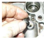
Lubrication Relief Valve: This valve is located in the side of the casting that houses the relief valve and consists of a plug, spring and ball as shown in the adjacent photos. The purpose of this valve is to provide an escape path for excess oil that can't be accepted by the lubrication system ---typically when running at high output RPM.
