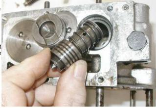
The right photo below shows a close up view of the valve and valve body. The hole in the valve body shows that the valve is about half open.
