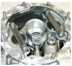
The operating piston diameter is 1.25 inches. The force exerted at 450 psi hydraulic pressure is:
