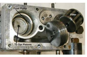
**Operating Pistons:** The operating pistons are located in the main casting as shown in the photo on right. The left piston has been removed. Note the rubber O-Rring used to seal the piston. The fluid entry and exit holes for the left cylinder are indicated on the photo.
