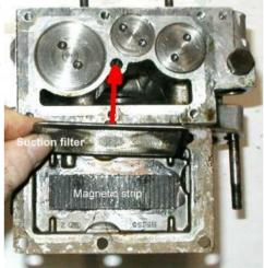
**The Pump:** The photo on the right shows the front of the main casting. The pump is in the lower part. The pump piston is pulled up and pushed down by the cam follower as the mainshaft and attached cam rotate. The pump piston, pin, cam and cylinder are steel. The Cam follower and the main casting are aluminum. The photo below shows the pump parts in more detail. From left to right:
