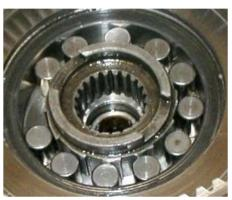
For counterclockwise rotation, the opposite is true. If the annulus is rotating slower than the mainshaft, the rollers go down the ramps and the clutch is released. If the annulus tries to rotate faster than the mainshaft, the rollers go up the ramp and lock the annulus to the mainshaft
