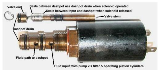
Relief Valve & Dashpot: The photo at right shows the dashpot and part of the relief valve being removed from the main casting. The plug was removed first and laid face up on the casting.
