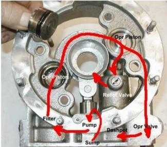
**Sump:** The bottom of the main casting is shown on the right. The sump cover has been removed with the inside surface face up. The magnetic strip is glued to the inside of the cover. The suction filter is identified. The filter is very thin and rests on the sump cover. The filter output is via a thin tube the fits into a hole in the main casting as shown by the red arrow. The high pressure filter, pump and the dashpot are accessed via the three plugs with small holes.
