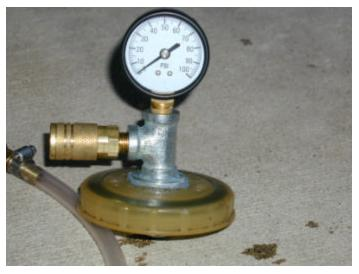
I used the quick connect setup to make it easier to take the cap on and off – in hind site I might have reversed the quick connect to keep the tank from leaking when we are all done.
