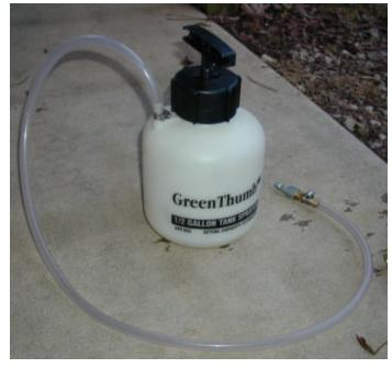
Take of the sprayer hose and attach some clear ¼ " tubing. At the end of the tubing attach a male quick connect coupling.
