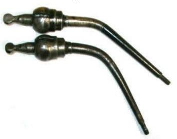
When the top cover was disassembled, signs that the 3<sup>rd</sup>/4<sup>th</sup> selector shaft been forced past the interlock were found. I suspect that someone tried to force the gearbox into reverse while it was still locked in 3<sup>rd</sup> or 4<sup>th</sup> either through the incorrectly set selector or the bent fork prong. It then went to work chewing up the reverse gear teeth.
